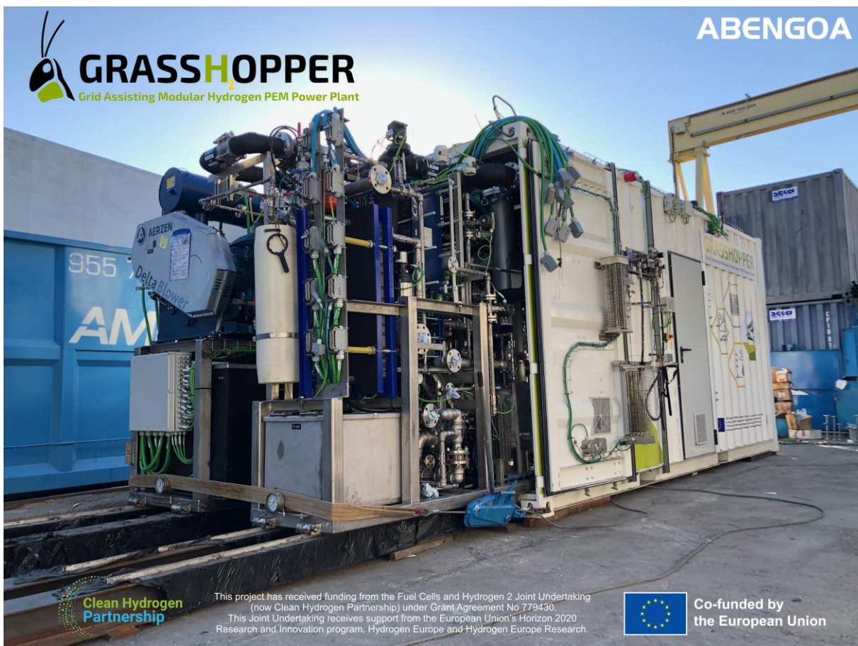
Figure 8– Finalisation of the construction phase for GRASSHOPPER pilot plant
