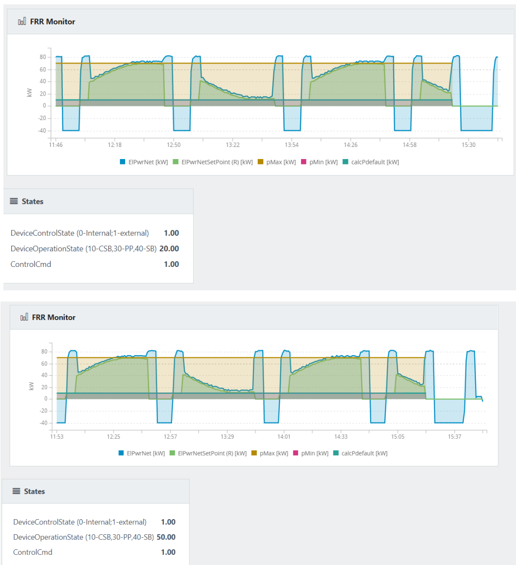
Figure 10: Changing of the Pnet and device operation state when stand by command executed
