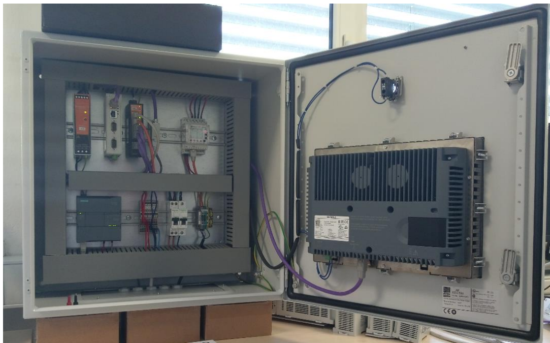
Figure 2: A generic FEMS – inside configuration.
